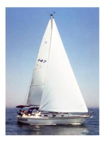
Shalom, a 1987 Pearson 36-2, is for sale. She is a comfortable cruiser (and occasional racer) and is offered in sailaway condition. *The underbody configuration is a keel-centerboard, drawing 4 2'with the board up and 8'3'with the board down. The L-shaped galley has a double sink, top-loading ice box, and propane stove and oven. The engine (replaced in 2002) is below the galley counter.*
